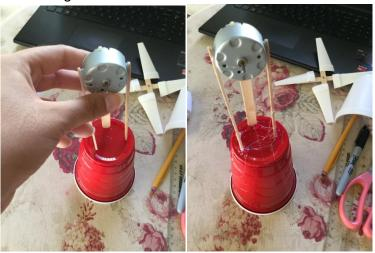
7. Attach the blades to the motor. The DC motor will be inserted into the hole on the cross-shaped base. After inserting it, secure it by hot gluing it.
